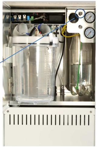
removed for filling. To re-install the bottle, align the threads on the bottle and the manifold and screw together. The bottle will be pressurised when the toggle switch is re-selected in the downwards direction. The clean water system also provides the mechanism for applying Biofilm removal process. Refer to the section on Biofilm removal.
