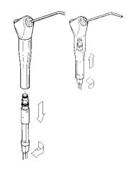
To install the syringe, slip the QD cartridge all the way into the syringe handle, then turn it clockwise a quarter turn until it stops. This will turn the air and water on, making the syringe operational.
